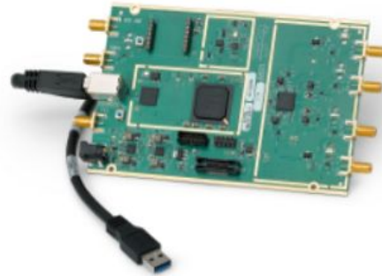
Figure 6:SDR B210 (Board Only)
